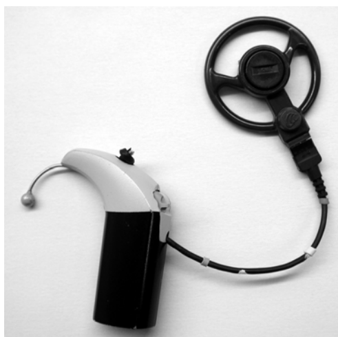
FIGURE 7. External part (ESPril™ 3G) of the Nucleus® 24 (Cochlear Ltd, Sydney, Australia) multichannel cochlear implant. The microphone and speech processor are in the behind-the-ear box and the external induction coil is fixed to the head with a magnet and sends the information to the internal coil.
