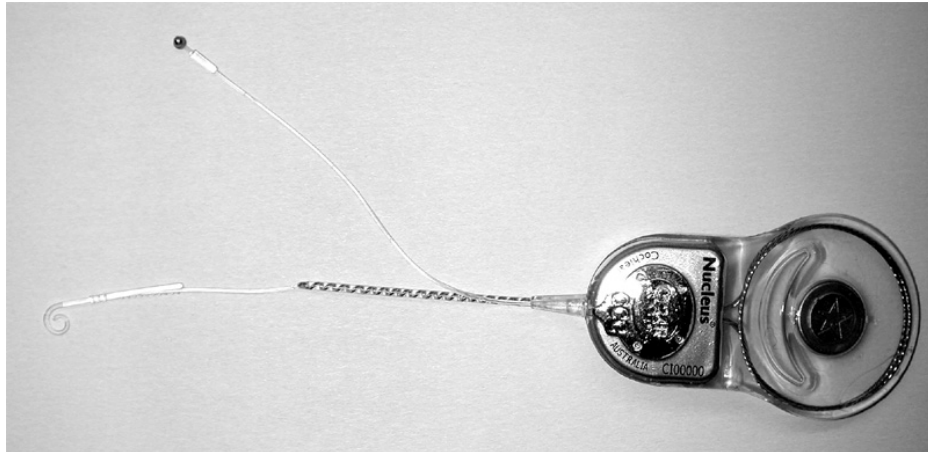
FIGURE 8. Internal part of the Nucleus® 24 Contour™ multichannel cochlear implant. The internal coil receives the information from the external coil. The titanium box contains the internal chip with the current sources. The curled electrode array is inserted in the cochlea and contains 22 electrodes and electrode contacts
